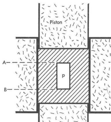
Fig. 11. Simplified model for piston-cylinder high pressure apparatus
