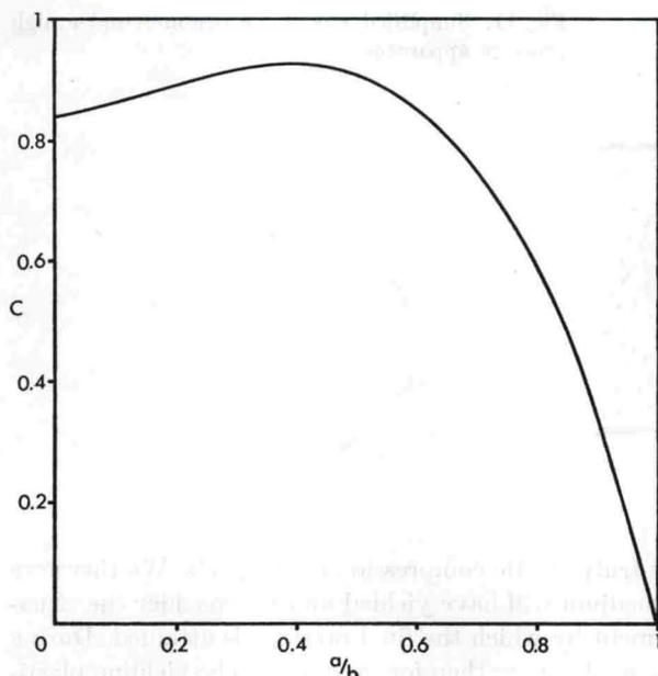
Fig. 12. Correction factor  $C$  as a function of diameter ratio  $a/b$
